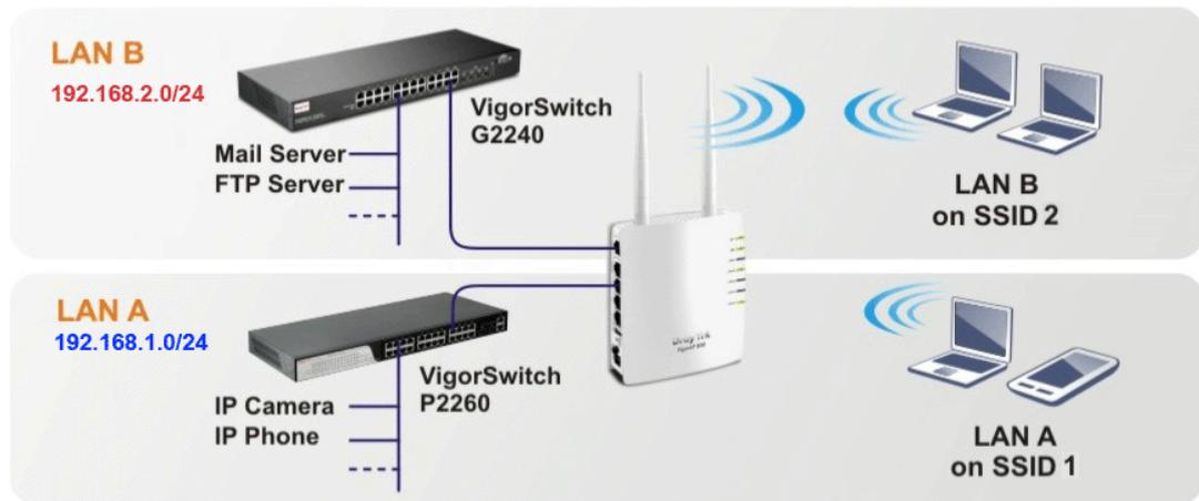
In the above figure, VigorAP 810 is used to control the wireless network connection. It can separate the wireless traffic between accessing internal server and the usage of video. Wireless station connecting to VigorAP 810 with SSID 2 can get the IP address with the network segment of 192.168.1.0/24 (LAN-A); wireless station connecting to VigorAP 810 with SSID 1 can get the IP address with the same network segment of 192.168.2.0/24 (LAN-B).
