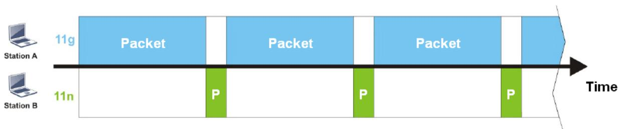
To improve this problem, Airtime Fairness is added for VigorAP 810. Airtime Fairness function tries to assign *similar airtime* to each station (A/B) by controlling TX traffic. In the following figure, Station B(11n) has higher probability to send data packets than Station A(11g). By this way, Station B(fast rate) gets fair airtime and it's speed is not limited by Station A(slow rate).
