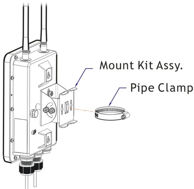
5. Press the pipe clamp to open it for clamping the pole.
