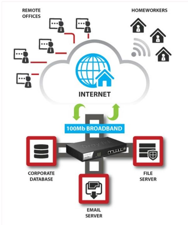
At the central site a high speed Vigor 2960 was installed to terminate the 100Mb/s broadband with 9 VPNs. With a 500 Mb/s capacity and the ability to terminate up to 200 VPN s this was a high quality solution with plenty of room for expansion.
