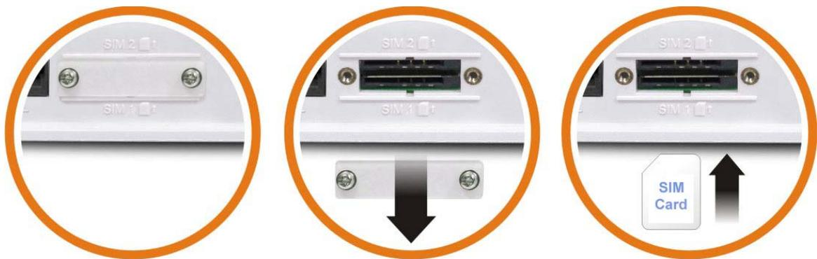
After installing the SIM card, fasten the back plate again.
