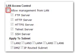
In the event that access to management is unavailable on LAN1, either change the LAN Access Control configuration by managing from the Internet, or downgrade to the previous firmware version with the DrayTek Firmware Upgrade utility to regain access via LAN1.
