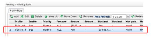
Now, any packets from LAN1 sent to the remote PC (IP address: 203.65.1.35) will be forcefully to pass through WAN1.
