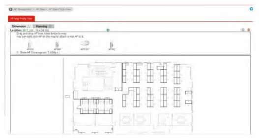
4. Check the box of **Show AP Coverage on** 5GHz/2.4 to display the signal coverage area.
