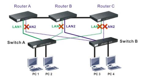
When LAN1 in Router A fails, one of the available line connections (e.g., LAN1 in Router C) will be selected to offer the network service for all the connected PCs.
