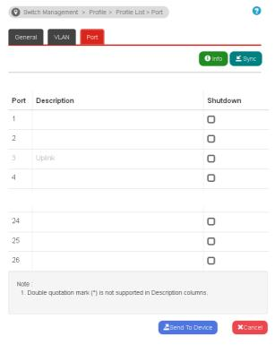
After finished the port configuration, click the VLAN tab to modify settings relevant to VLAN.
