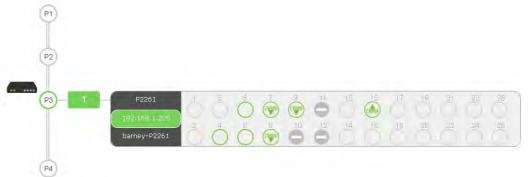
**Note**: If the hierarchy display is incorrect, please access into the web user interface of VigorSwitch and enable the function of LLDP (e.g., Configuration >>DDLP>>LLDP General Setup in VigorSwitch 2261). The interval for LLDP shall be less than 3 minutes (the default setting, 30 seconds).
