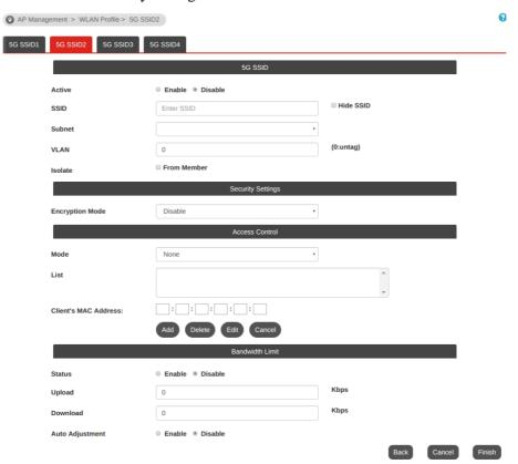
5. When you finished the above web page configuration, click **Finish** to exit and return to the first page. The modified WLAN profile will be shown on the web page.
