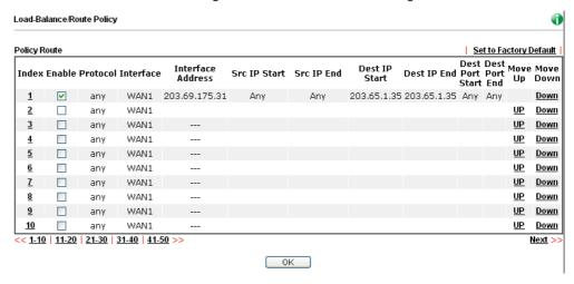
Now, the packets sent to the remote PC (IP address: 203.65.1.35) will be forced to pass through WAN1.
