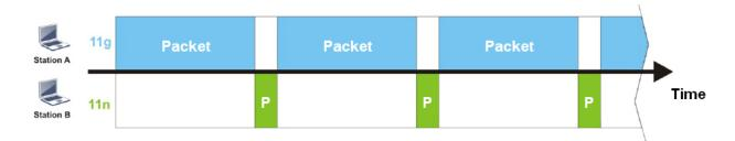
To improve this problem, Airtime Fairness is added for Vigor router. Airtime Fairness function tries to assign *similar airtime* to each station (A/B) by controlling TX traffic. In the following figure, Station B(11n) has higher probability to send data packets than Station A(11g). By this way, Station B(fast rate) gets fair airtime and it's speed is not limited by Station A(slow rate).
