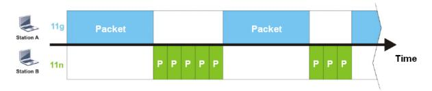
It is similar to automatic Bandwidth Limit. The dynamic bandwidth limit of each station depends on instant active station number and airtime assignment. Please note that Airtime
