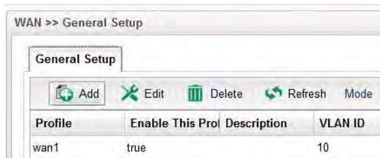
5. Create a new WAN profile named with **wan1\_1**, and set VLAN ID named with **111** based on WAN Port 1(WAN1). Note that **Untag** must be set with **Disable**. It means wan1\_1 can accept the packets tagged with VLAN ID 111. Next, click **Apply** to save the settings.
