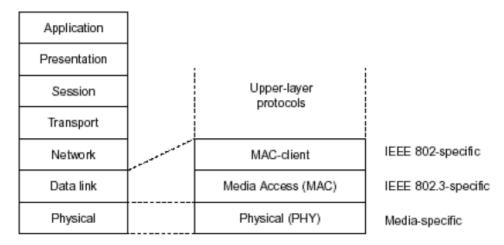
In the above figure, we can see that Ethernet locates at the Data Link layer and Physical layer and comprises three portions, including logical link control (LLC), media access control (MAC), and physical layer. The first two comprises Data link layer, which performs splitting data into frame for transmitting, receiving acknowledge frame, error checking and re-transmitting when not received correctly as well as provides an error-free channel upward to network layer.
