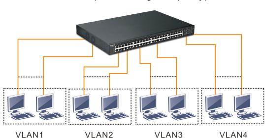
Case 2: Port-based VLAN -1 (\*The switch image is sample only.)
